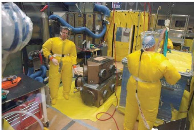
*Contact-Handled Waste is processed in an airlock room*
