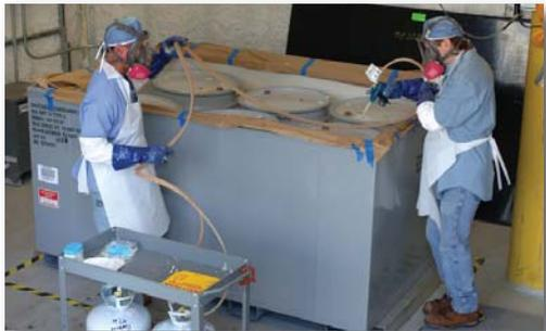
Applying foaming agents to Mixed Low-Level Waste drums in macroencapsulation boxes for safe transport to the Nevada Test Site for disposal
