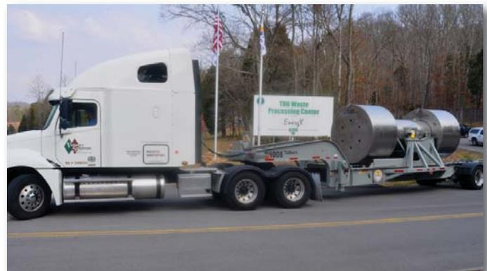
RH-72B Shipping Cask used in transporting Remote-Handled TRU Waste departs the TRU Waste Processing Center for WIPP.
